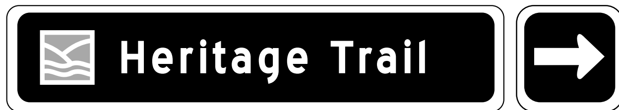
3 Sign Type C1-3 - Horizontal End of the exit ramp, 6" type Note: Arrow direction changes sides and direction as determined by its location
